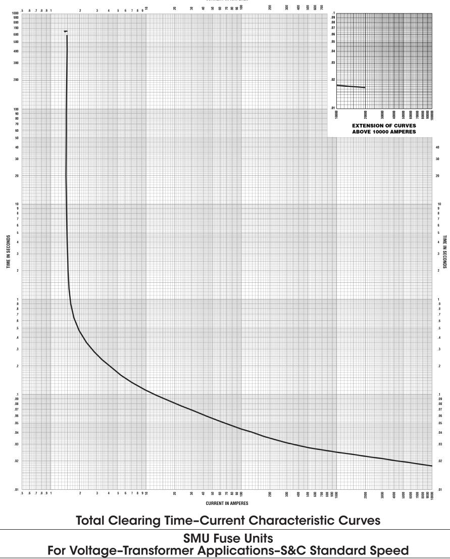
BASIS—These fuse units are tested in accordance with the procedures described in IEEE Standard C37.41. As required by this standard, the minimum melting curve and total clearing curves are based on tests starting with the fuse unit at an ambient temperature of 25°C (77°F) and no initial load.
